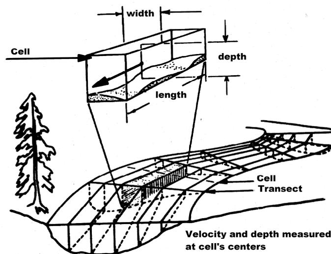
Figure 6: Curvilinear 1D PHABSIM discretisation scheme for characterizing abiotic factors
